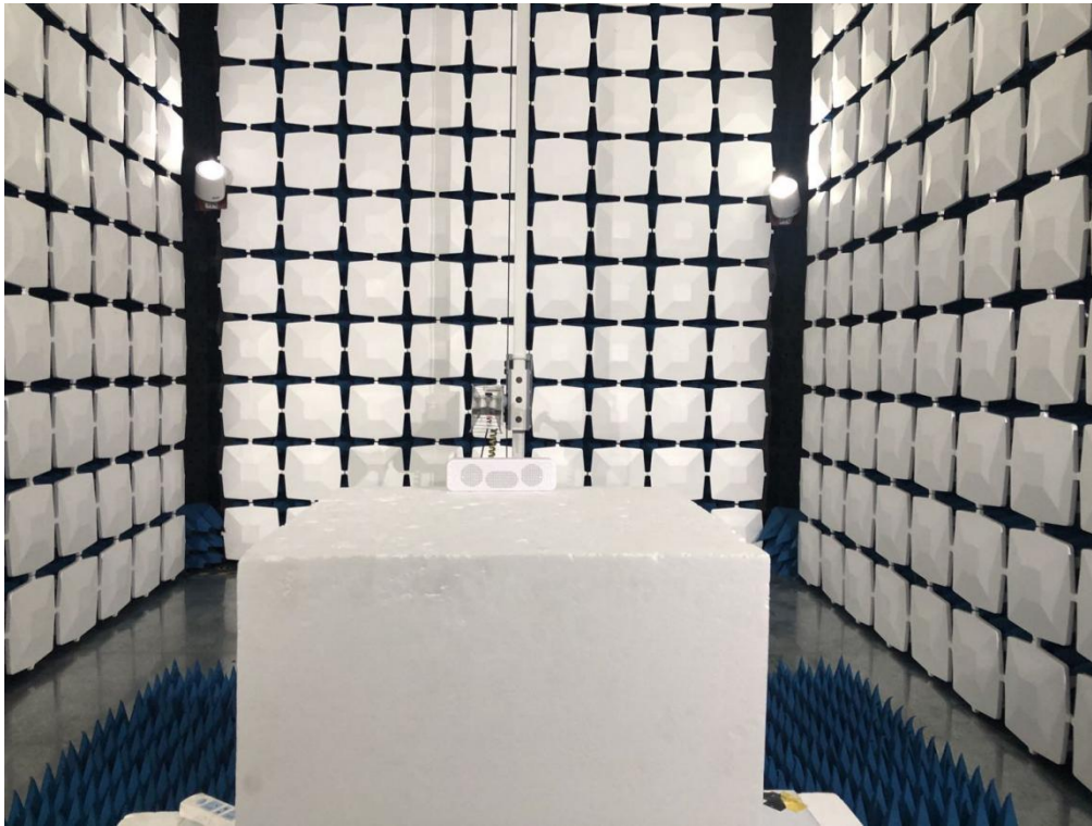
Above 1GHz for radiated emission test setup
