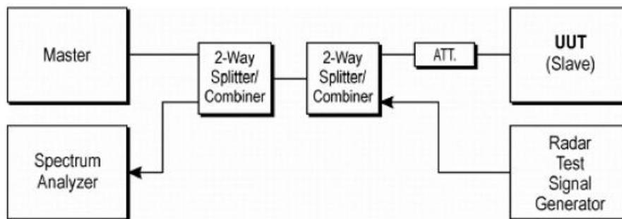
Figure 3-1. Conducted Test Setup for DFS
