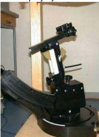
Larger DUT's (e.g. notebooks) cannot be tested using this device holder. Instead a support of bigger polystyrene cubes and thin polystyrene plates is used to position the DUT in all relevant positions to find and measure spots with maximum SAR values. Therefore those devices are normally only tested at the flat part of the SAM.
