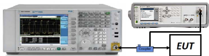
Figure 7-5. Test Instrument & Measurement Setup
