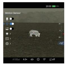
tilt angle appears on the left side of the screen and the pitch angle appears on the right side of the screen.
