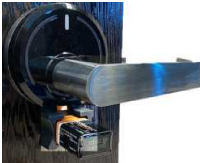
Emergency Battery Pack connected to rosette
