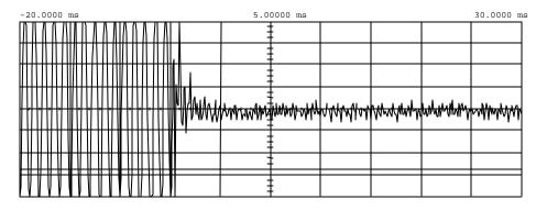
Trigger mode : Edge On Negative Edge Of Chan2 Trigger Level Chan2 = -27.500 mV (noise reject ON) Holdoff = 40.000 ns
