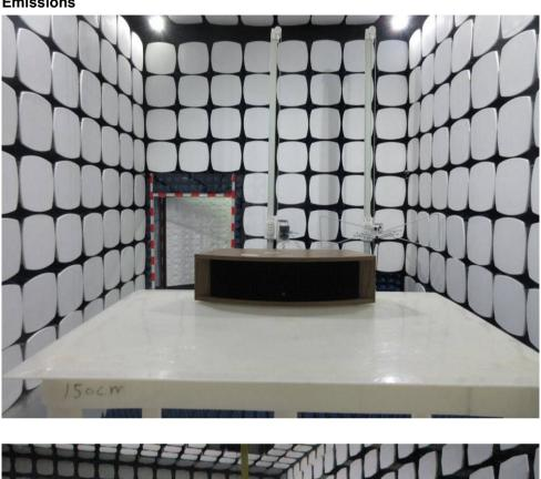
Radiated Emissions which fall in the restricted bands & Radiated Spurious **Emissions**
