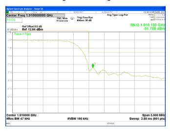
A8 FIELD STRENGTH OF SPURIOUS RADIATION MEASUREMENT GSM 850: (30-9000)MHz
