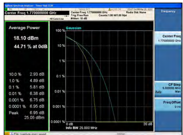
Band66 / 20MHz / High CH / 16QAM
