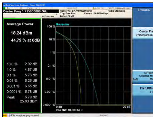
Band66 / 10MHz / Mid CH / 16QAM
