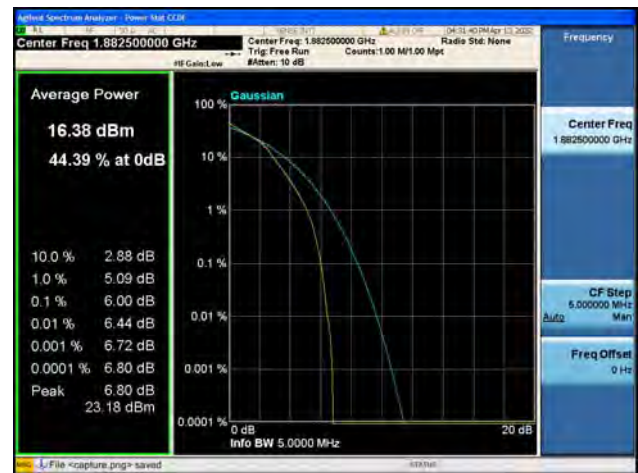
Band25 / 3MHz / High CH / 16QAM
