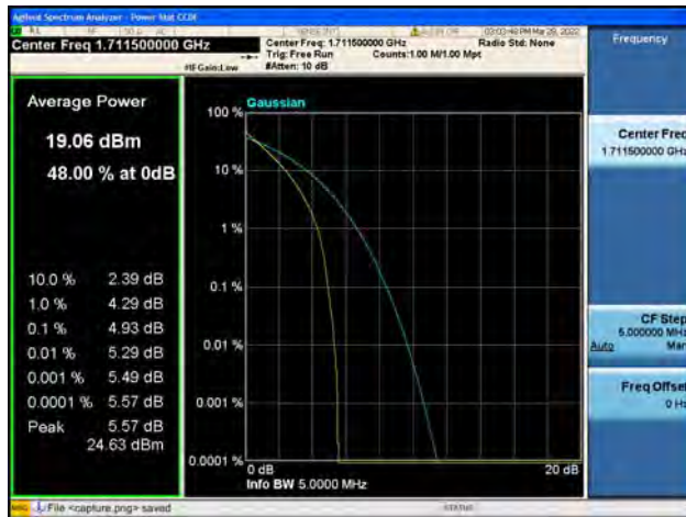
Band66 / 3MHz / Mid CH / QPSK
