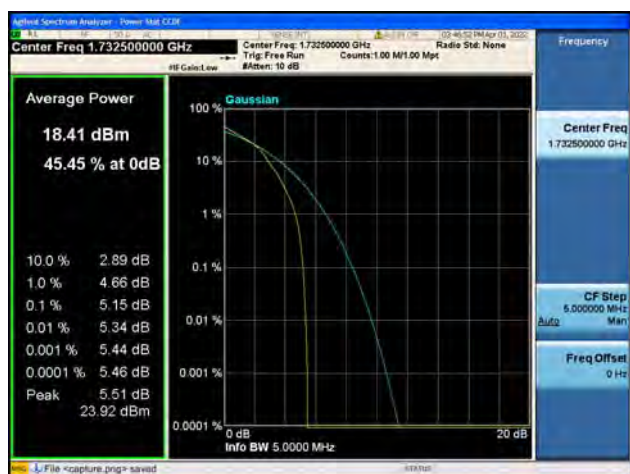
Band4 / 1.4MHz / High CH / 16QAM
