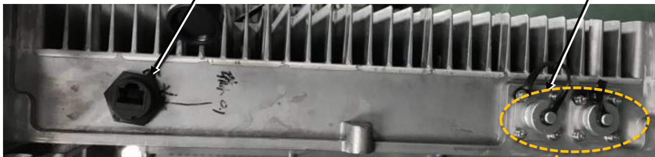
DRY CONTACT (8 pin) and external alarm interface (6pin)
