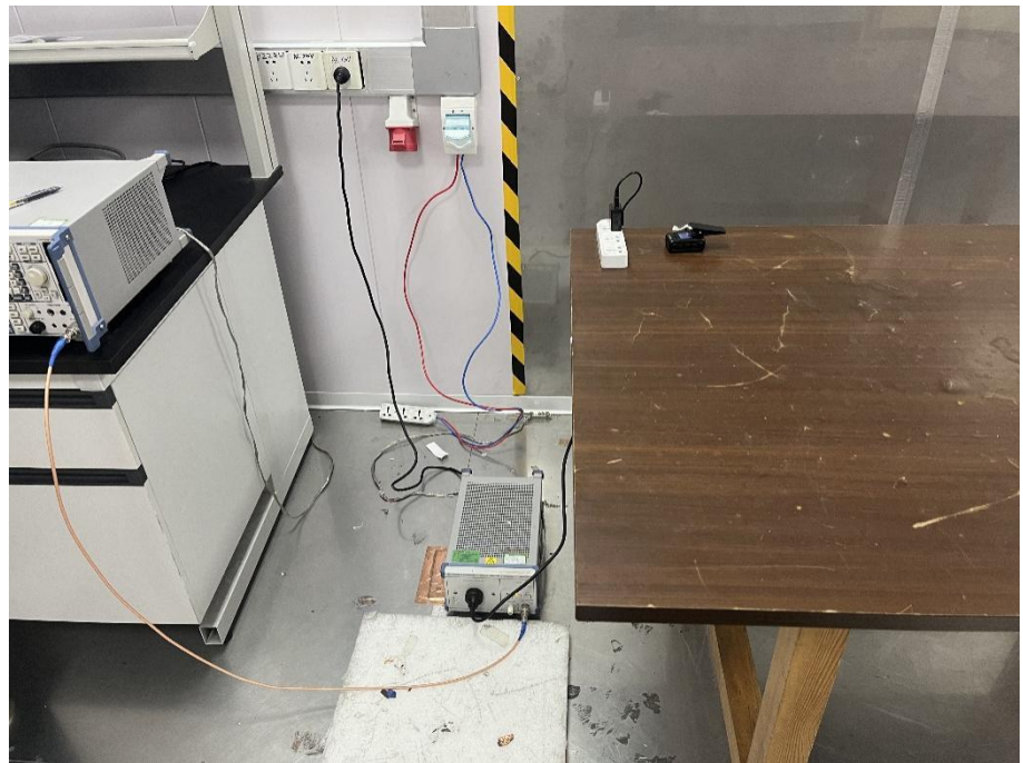
Conducted Emission Test Setup
