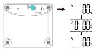
5. How to turn off the buzzer:Press and hold the UNIT button on the back for more than 2 seconds to switch the switch state, 1 sound means turn off the buzzer, 2 sounds means turn on the buzzer.The buzzer will sound 1 time to turn off the buzzer and 2 times to turn on the buzzer.
