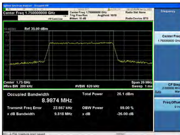
Band4 / 10MHz / High CH / 16QAM
