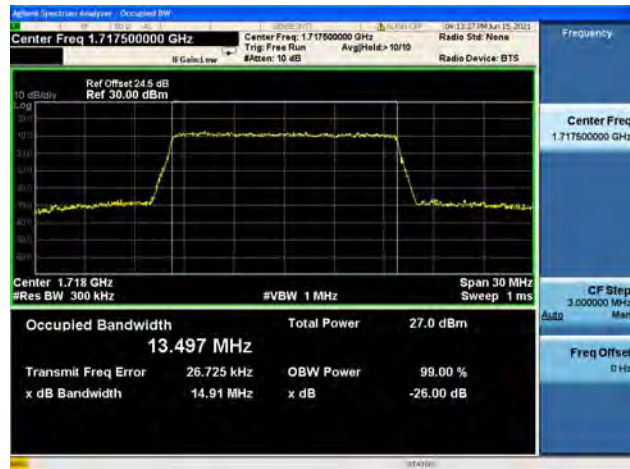
Band66 / 15MHz / Low CH / 64QAM
