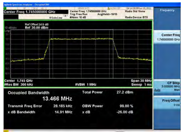
Band66 / 15MHz / Mid CH / 64QAM
