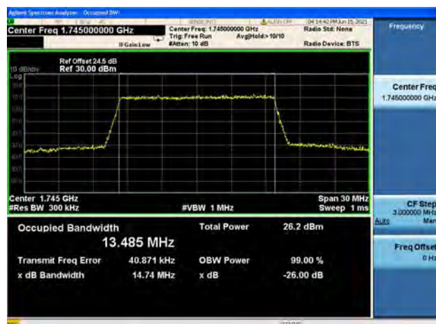
Band66 / 15MHz / Mid CH / 16QAM
