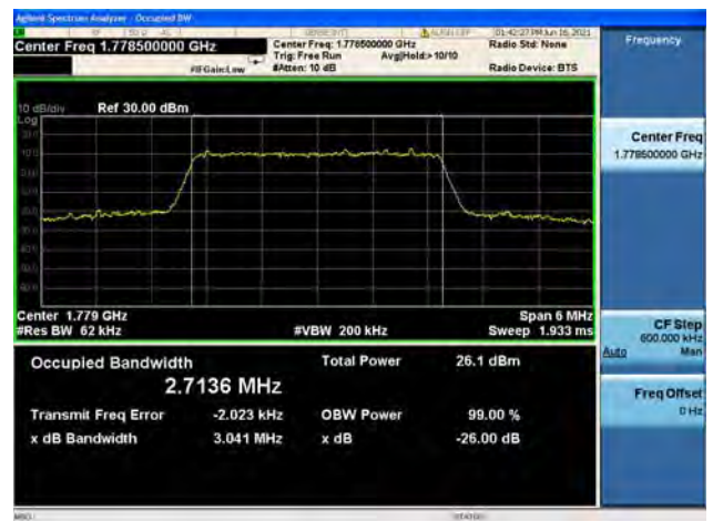
Band66 / 3MHz / High CH / 64QAM
