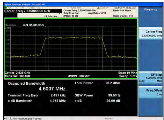
Band7 / 5MHz / Mid CH / 64QAM
