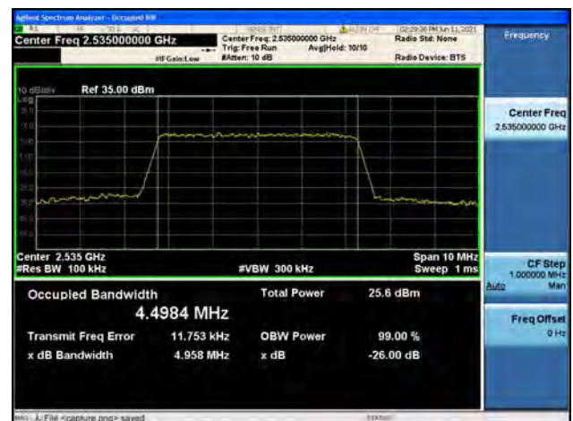
Band7 / 5MHz / Mid CH / 64QAM
