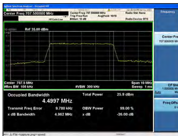
Band12 / 5MHz / Mid CH / 64QAM
