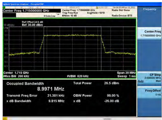
Band66 / 10MHz / Low CH / 64QAM
