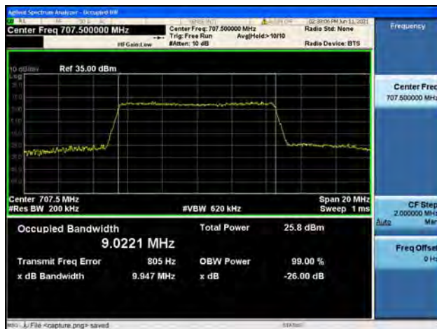
Band12 / 10MHz / High CH / 16QAM
