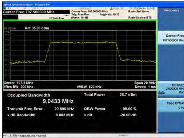
Band12 / 10MHz / Mid CH / 64QAM
