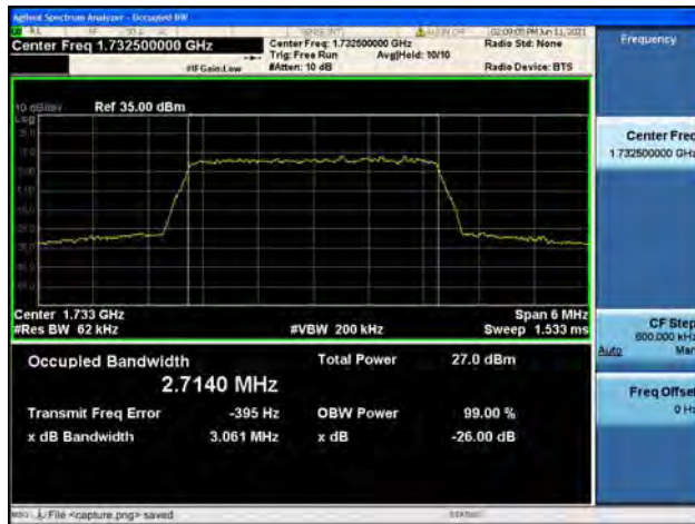
Band4 / 3MHz / Mid CH / 64QAM
