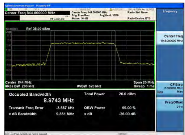
Band5 / 10MHz / High CH / 64QAM
