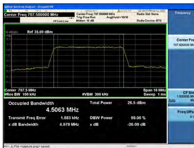
Band12 / 5MHz / Mid CH / 64QAM
