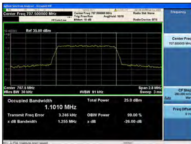
Band12 / 1.4MHz / Mid CH / 16QAM
