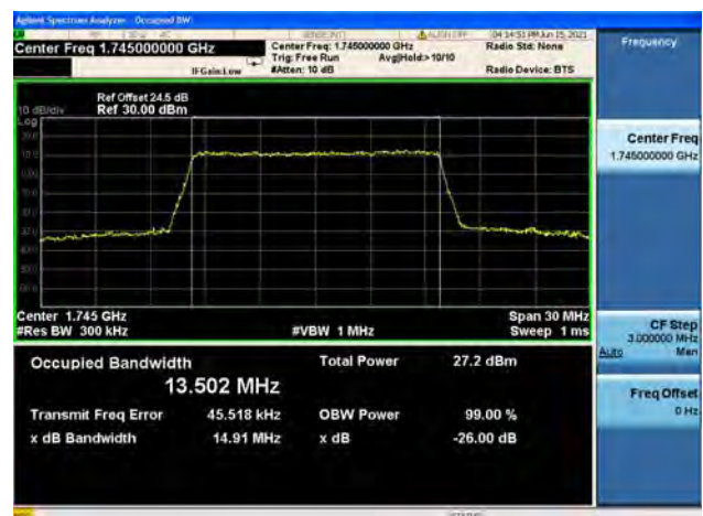
Band66 / 15MHz / Mid CH / 64QAM
