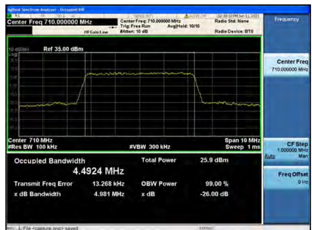
Band17 / 5MHz / Mid CH / 64QAM
