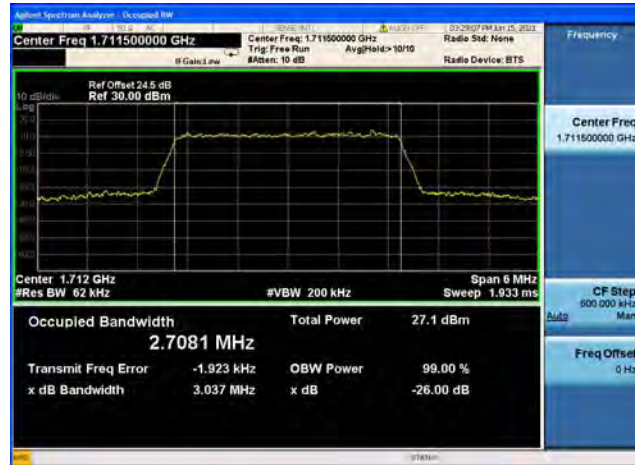
Band66 / 3MHz / Low CH / 64QAM
