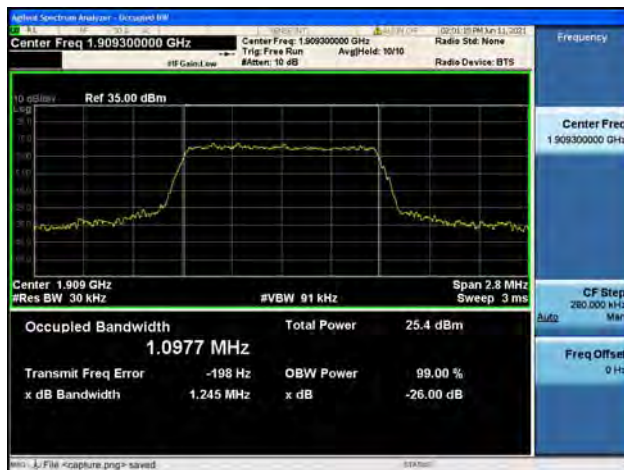
Band2 / 3MHz / Low CH / 16QAM
