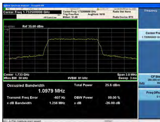
Band4 / 1.4MHz / Mid CH / 64QAM
