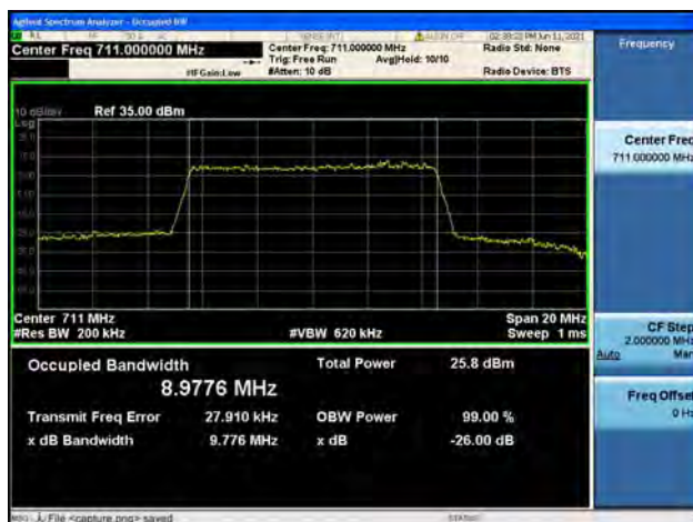
Band12 / 10MHz / High CH / 16QAM
