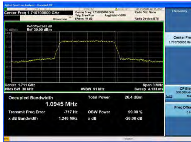
Band66 / 1.4MHz / Low CH / 64QAM
