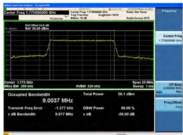
Band66 / 10MHz / High CH / 64QAM
