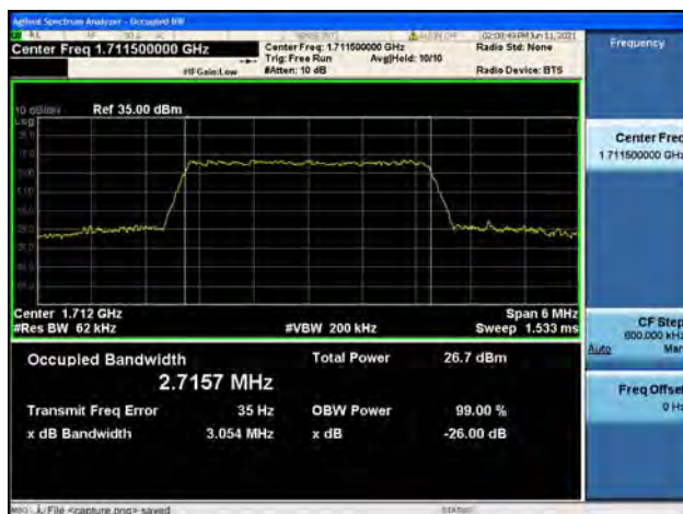
Band4 / 3MHz / Low CH / 16QAM
