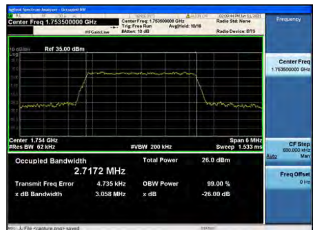
Band4 / 3MHz / High CH / 64QAM
