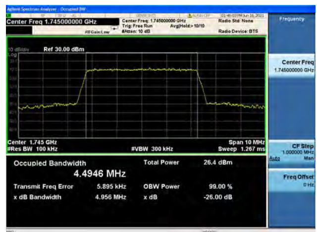
Band66 / 5MHz / Mid CH / 64QAM
