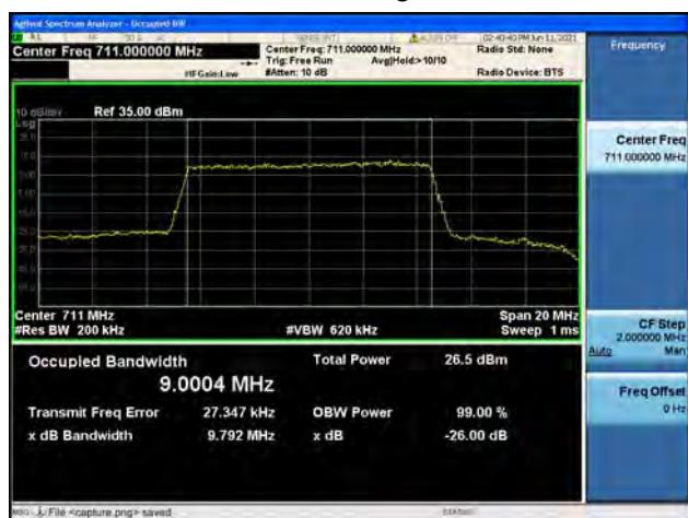
Band17 / 10MHz / High CH / 64QAM
