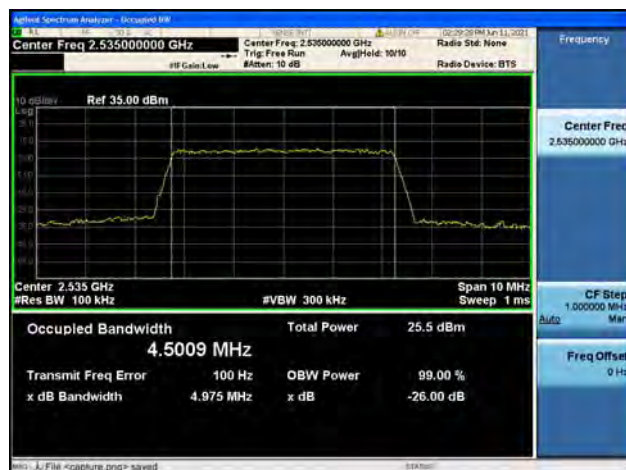
Band7 / 5MHz / Mid CH / 16QAM
