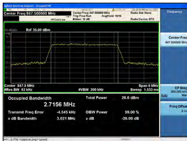
Band5 / 3MHz / High CH / 16QAM
