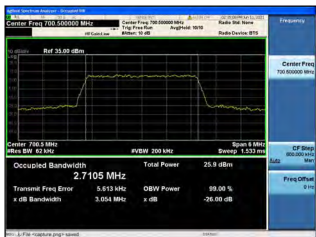
Band12 / 3MHz / Low CH / 16QAM
