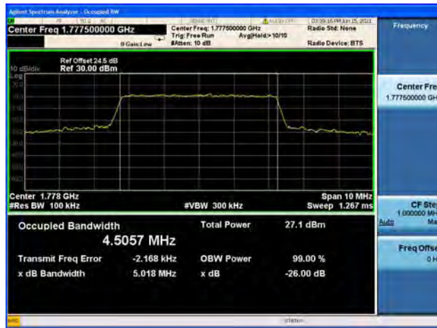
Band66 / 5MHz / High CH / 64QAM
