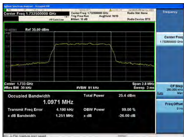
Band4 / 1.4MHz / Mid CH / 16QAM
