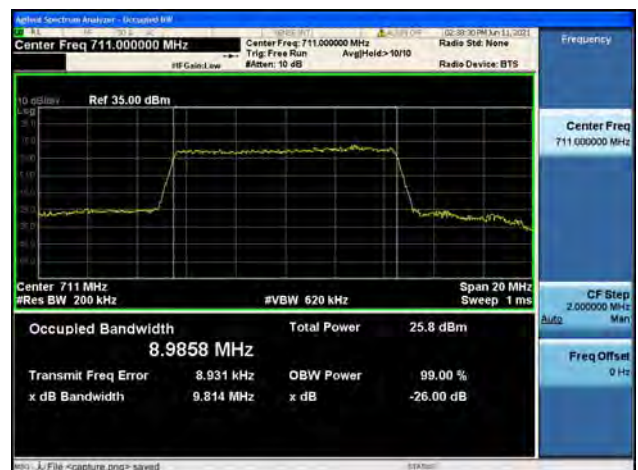
Band12 / 10MHz / High CH / 64QAM
