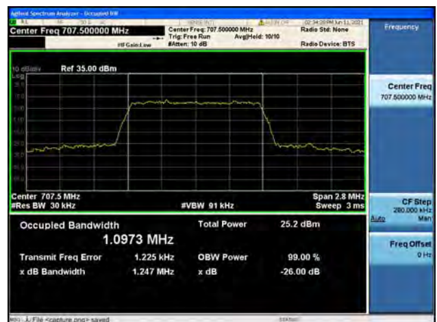
Band12 / 1.4MHz / Mid CH / 64QAM
