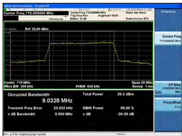
Band17 / 10MHz / Mid CH / 64QAM
