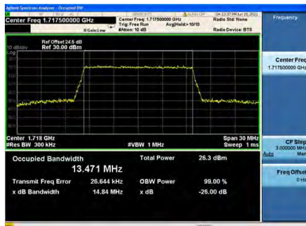
Band66 / 15MHz / Mid CH / 16QAM
