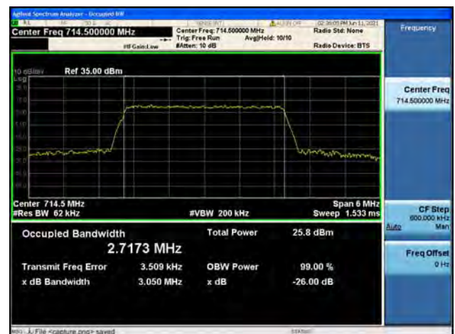
Band12 / 3MHz / High CH / 64QAM
