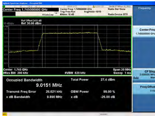
Band66 / 10MHz / Mid CH / 64QAM
