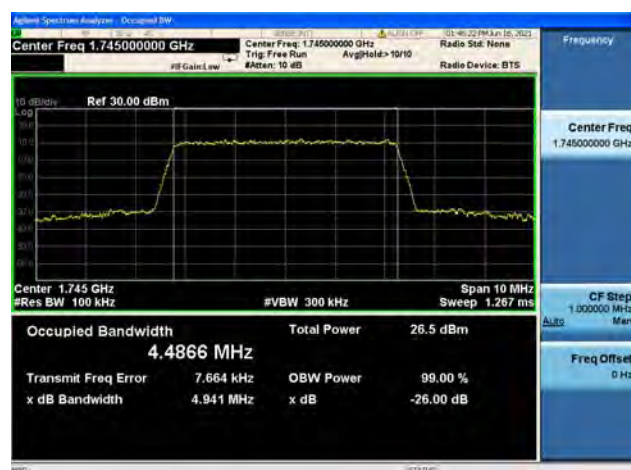
Band66 / 5MHz / Mid CH / 16QAM
