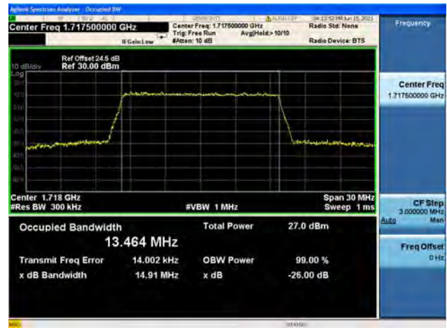
Band66 / 15MHz / Mid CH / QPSK
