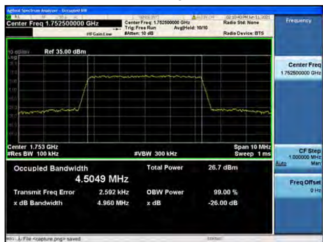
Band4 / 5MHz / High CH / 64QAM
