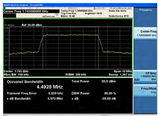
Band66 / 5MHz / Mid CH / 64QAM
