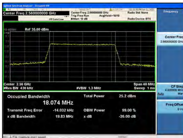
Band7 / 20MHz / High CH / 16QAM
