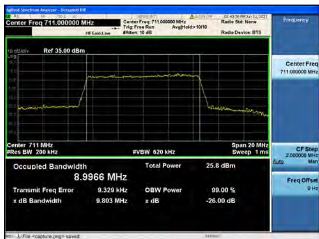
Band17 / 10MHz / High CH / 64QAM
