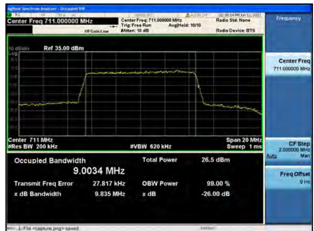
Band12 / 10MHz / High CH / 64QAM
