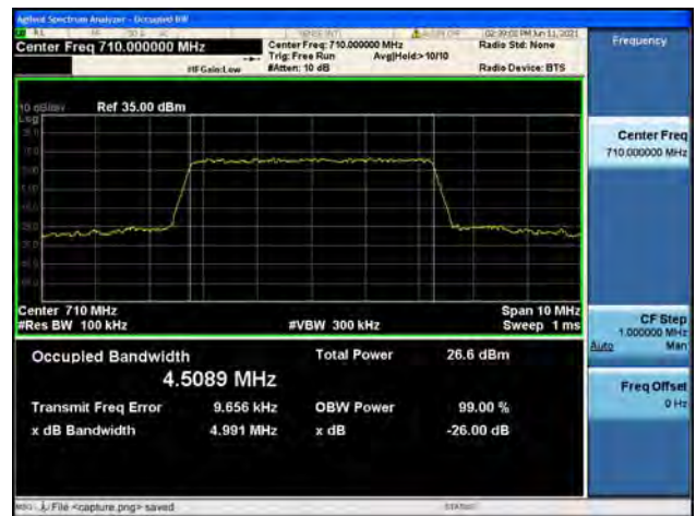
Band17 / 5MHz / Mid CH / 64QAM
