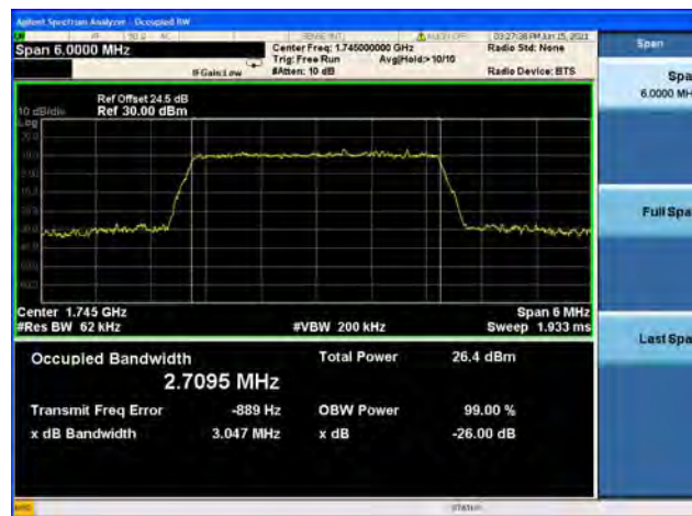
Band66 / 3MHz / High CH / 16QAM
