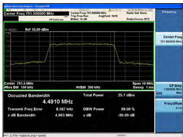
Band12 / 5MHz / Mid CH / 16QAM
