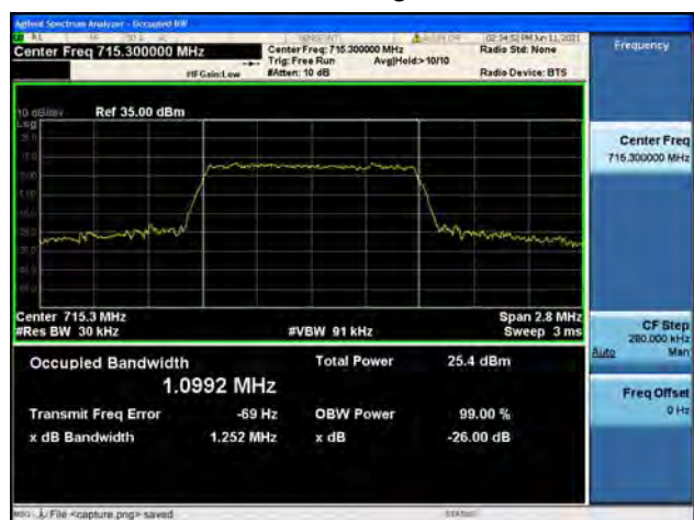
Band12 / 3MHz / Low CH / 16QAM
