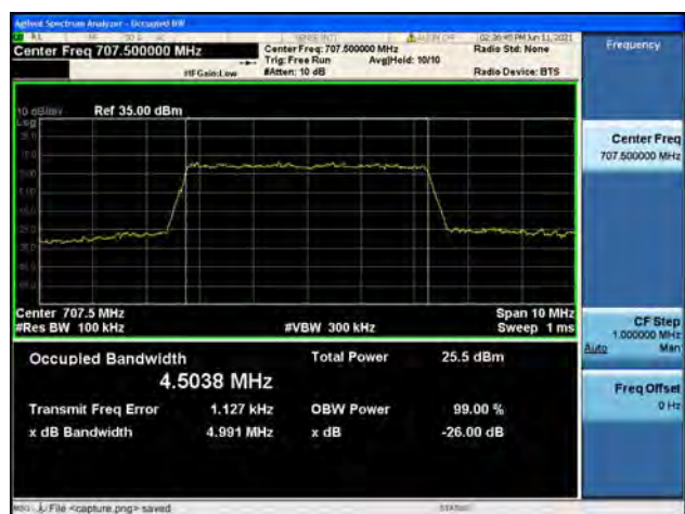
Band12 / 5MHz / Mid CH / 16QAM
