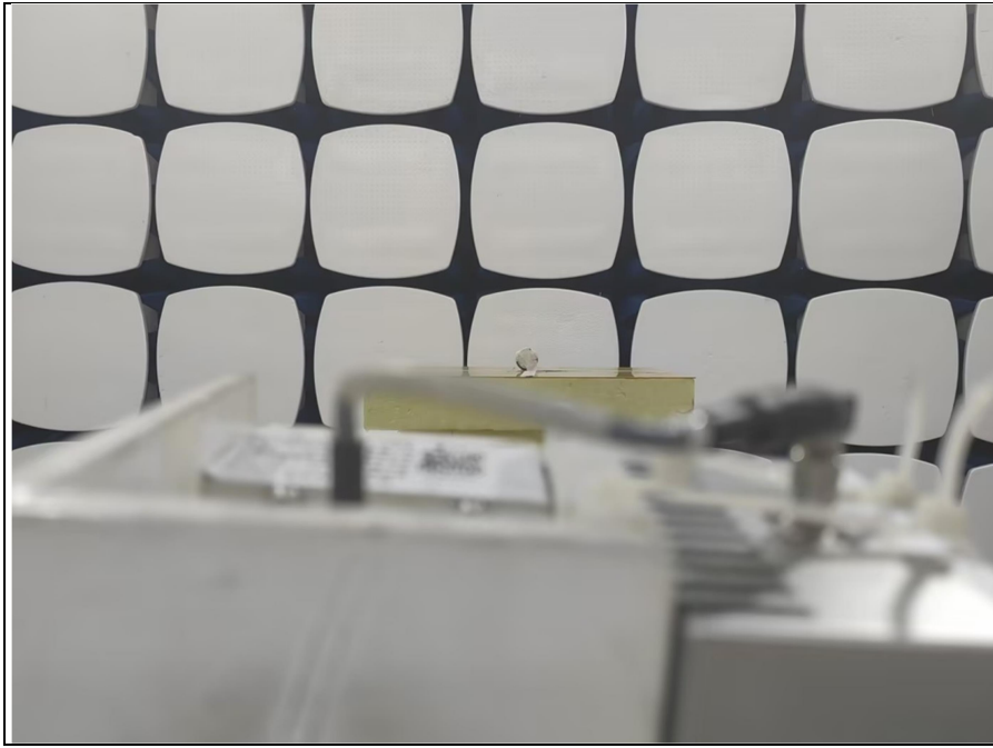
Radiated spurious emissions at frequencies above 18GHz
