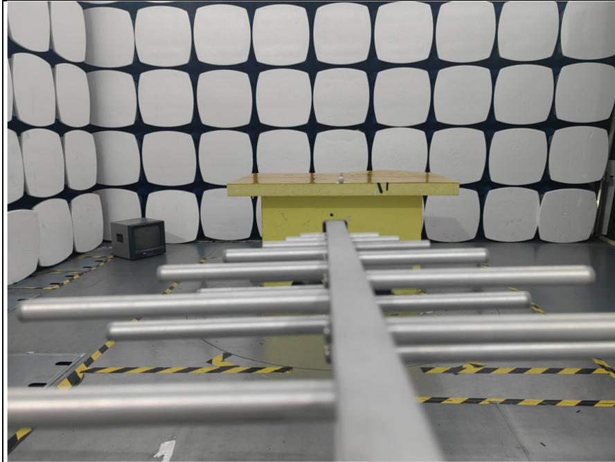
Radiated spurious emissions at frequencies up to 1 GHz
