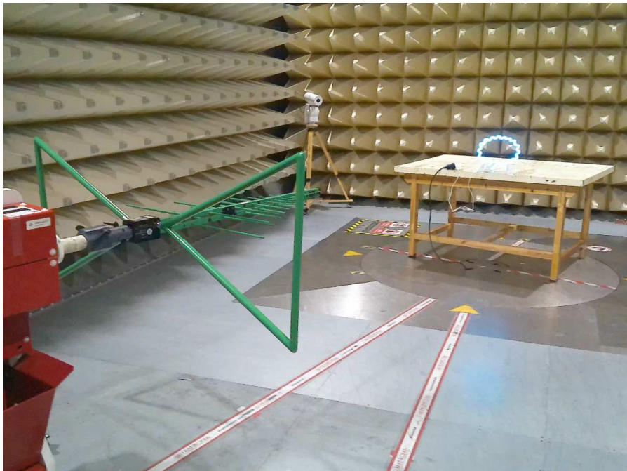
Photograph 2: Set-up for measurement of radiated emission
