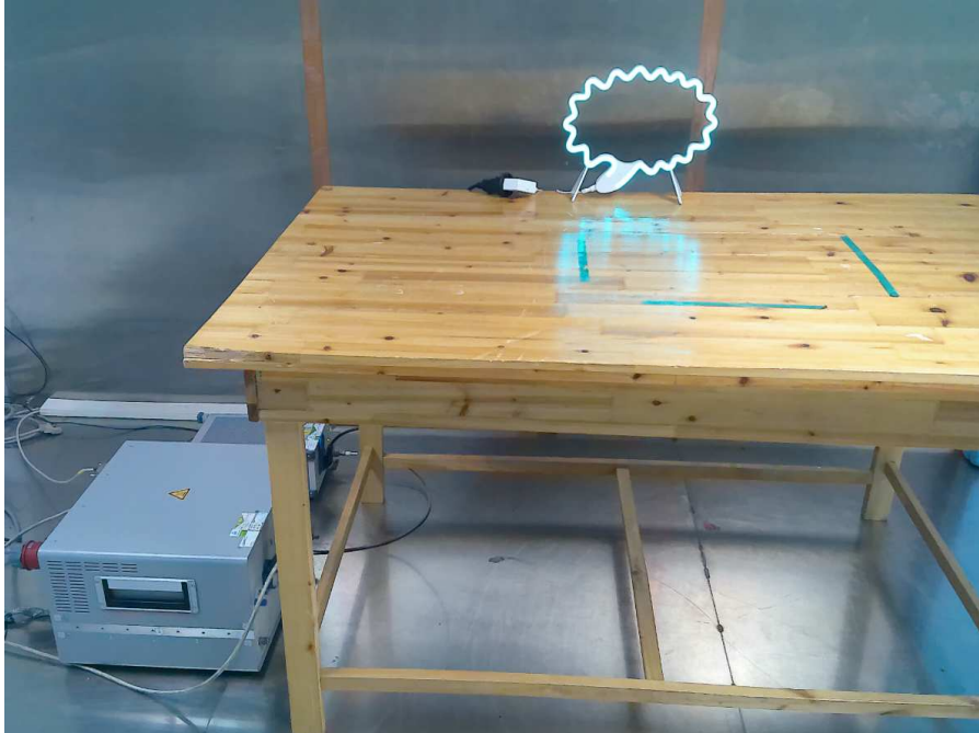
Photograph 2: Set-up for measurement of radiated emission
