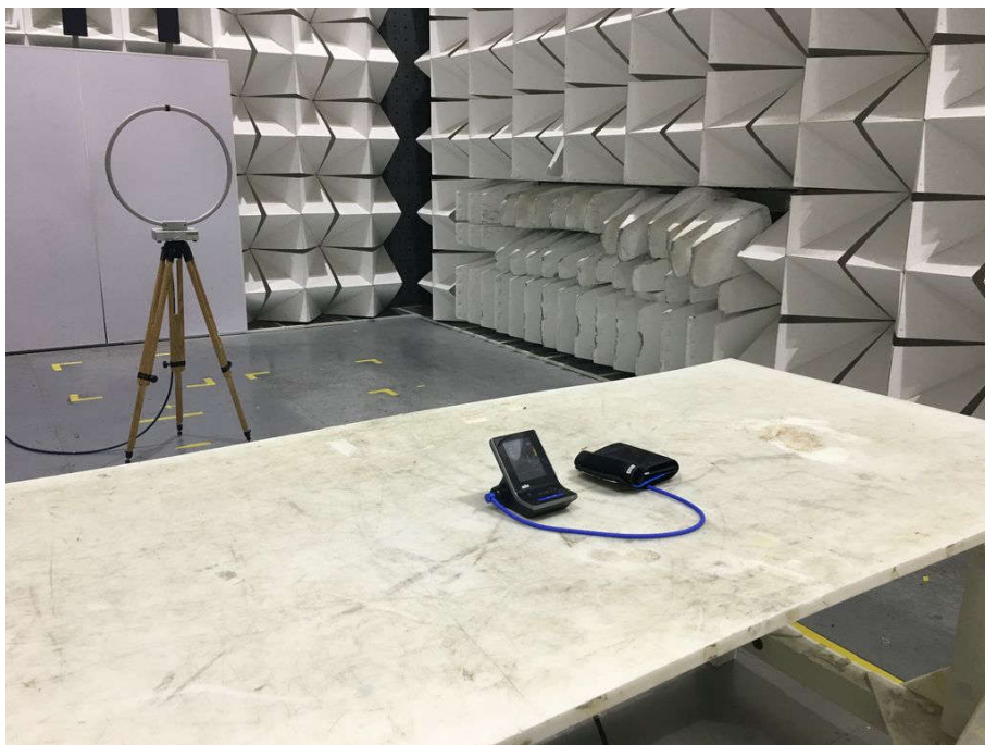
Radiated spurious emission Test Setup-1(Below 30MHz)
