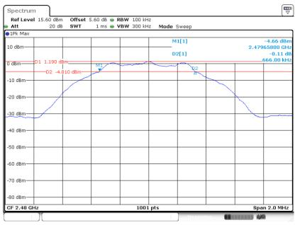
6 dB Bandwidth Plot on Channel 39
