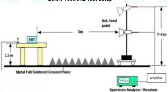
**Above 1GHz Test Setup**
