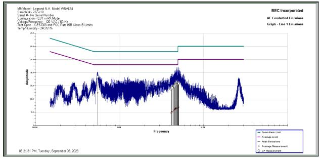
**Results:** All conducted emissions measured on the AC Power Port of the Legrand Model WNAL34 Sample 2272-10 in Rx Mode are below the limit specified by FCC Part 15.207 and RSS-Gen 7.2 Limits by a margin of 19.11 dB.
