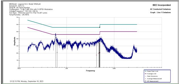
**Results:** All conducted emissions measured on the AC Power Port of the Legrand Model WNAL44 Sample 2272-12 in Tx Mode Middle Channel at 2.440 GHz are below the limit specified by FCC Part 15.207 and RSS-Gen 7.2 Limits by a margin of 12.06 dB.
