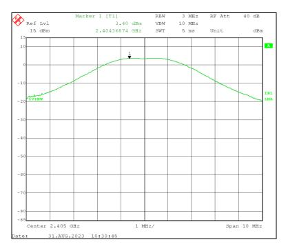
Legrand Model WNAL34 with Zigbee Radio Middle Channel 18, 2.440 GHz, O-QPSK Modulation
