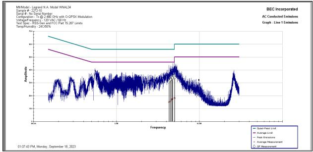
**Results:** All conducted emissions measured on the AC Power Port of the Legrand Model WNAL34 Sample 2272-10 in Tx Mode High Channel at 2.480 GHz are below the limit specified by FCC Part 15.207 and RSS-Gen 7.2 Limits by a margin of 19.45 dB.
