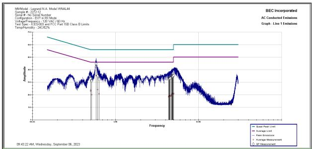
**Results:** All conducted emissions measured on the AC Power Port of the Legrand Model WNAL44 Sample 2272-12 in Rx Mode are below the limit specified by FCC Part 15.207 and RSS-Gen 7.2 Limits by a margin of 11.34 dB.
