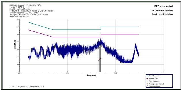
**Results:** All conducted emissions measured on the AC Power Port of the Legrand Model WNAL34 Sample 2272-10 in Tx Mode Low Channel at 2.405 GHz are below the limit specified by FCC Part 15.207 and RSS-Gen 7.2 Limits by a margin of 16.73 dB.
