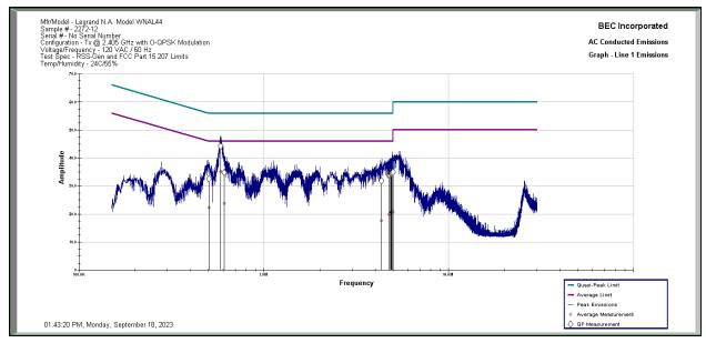
**Results:** All conducted emissions measured on the AC Power Port of the Legrand Model WNAL44 Sample 2272-12 in Tx Mode Low Channel at 2.405 GHz are below the limit specified by FCC Part 15.207 and RSS-Gen 7.2 Limits by a margin of 10.78 dB.
