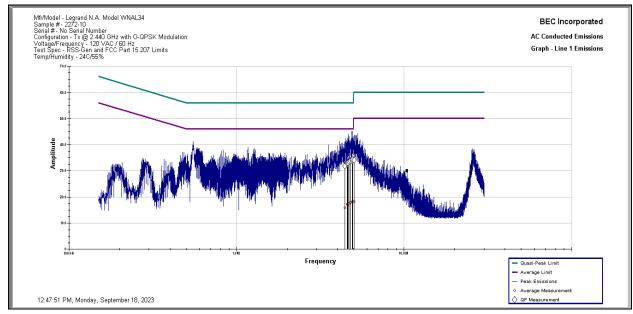
**Results:** All conducted emissions measured on the AC Power Port of the Legrand Model WNAL34 Sample 2272-10 in Tx Mode Middle Channel at 2.440 GHz are below the limit specified by FCC Part 15.207 and RSS-Gen 7.2 Limits by a margin of 19.48 dB.
