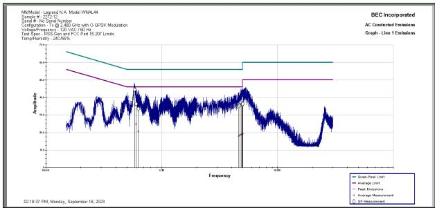
**Results:** All conducted emissions measured on the AC Power Port of the Legrand Model WNAL44 Sample 2272-12 in Tx Mode High Channel at 2.480 GHz are below the limit specified by FCC Part 15.207 and RSS-Gen 7.2 Limits by a margin of 10.52 dB.
