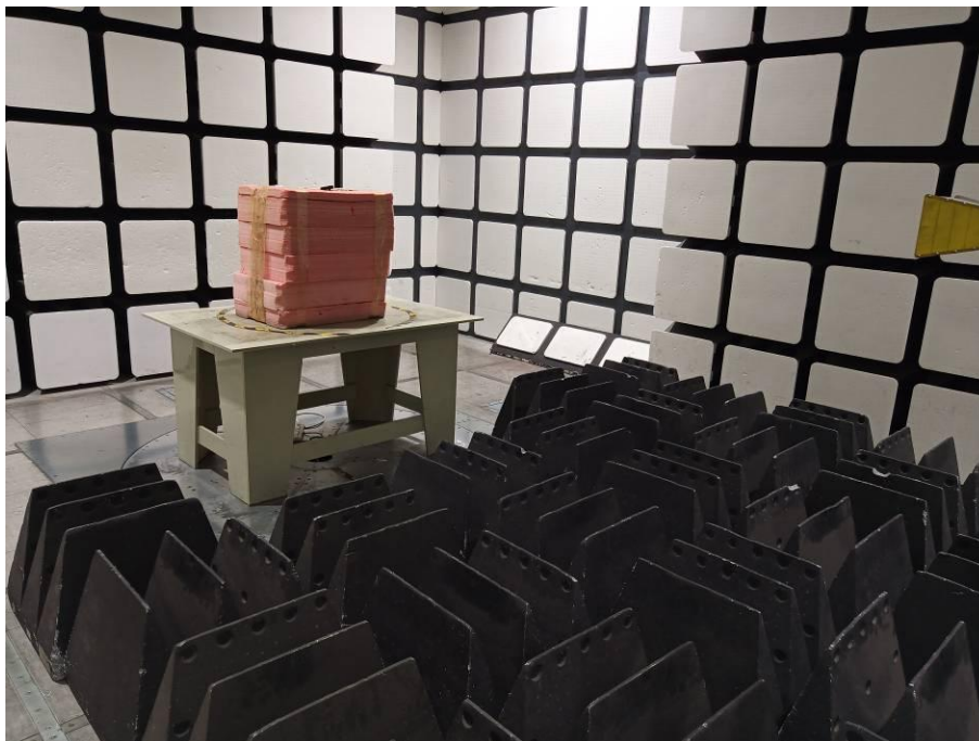
Radiated Emissions View (Above 1 GHz)
