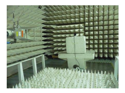
Photograph No.4 Setup for OBW, emission mask measurements
