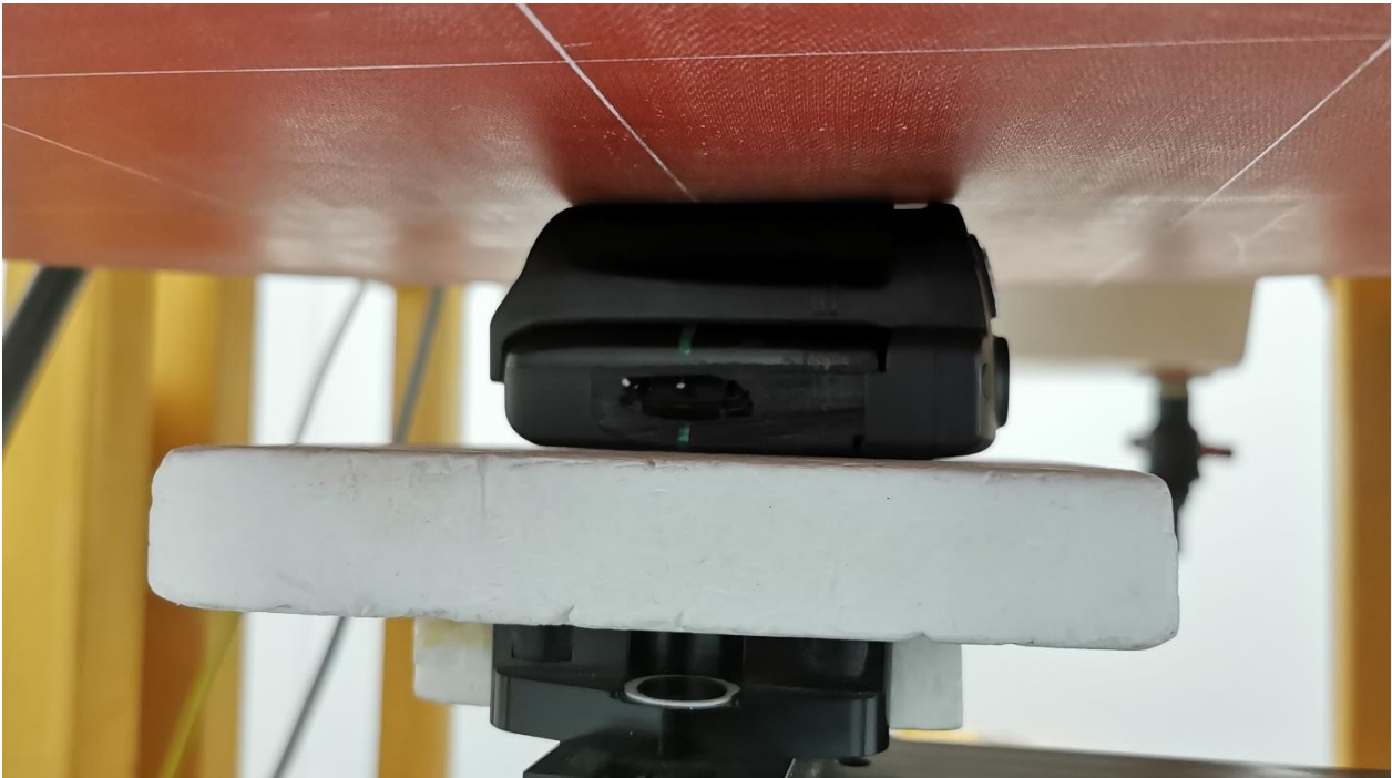
Figure 7. Front side of the DUT, SOLO 3 Portable Charger (SPC), 0mm
