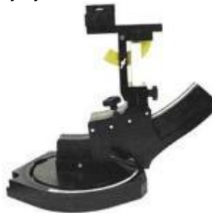
Device holder supplied by SPEAG
