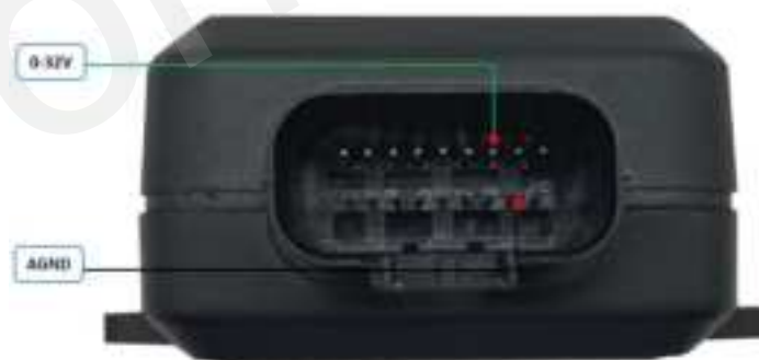
Figure 10. Typical Analogue Input Connection
