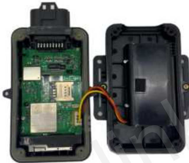
Figure 6. Backup Battery Installation
