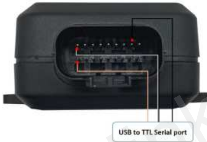
Figure 17. Typical Connection with USB to TTL Serial Port
