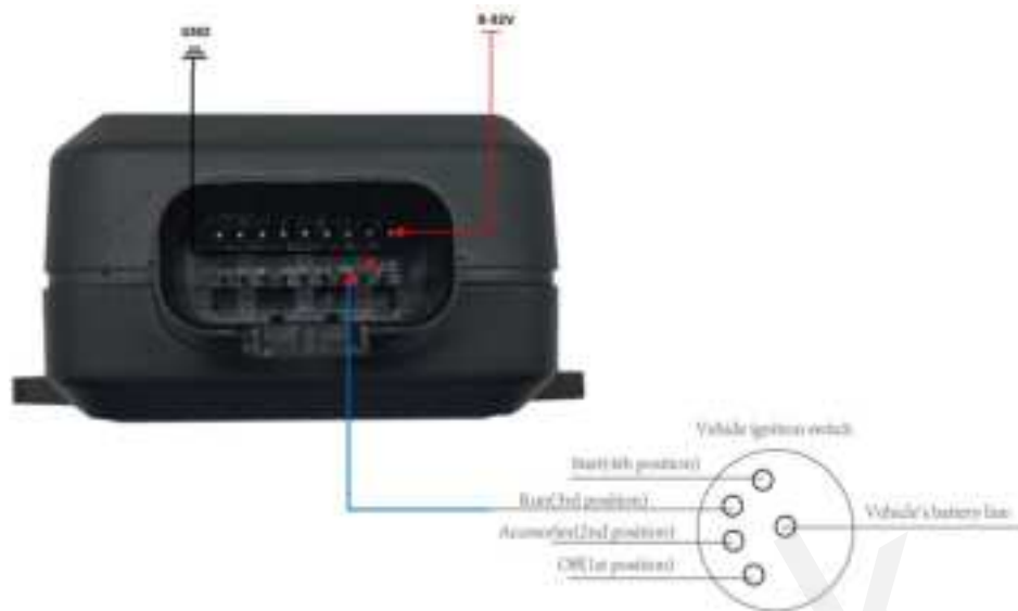
Figure 8. Typical Ignition Detection
