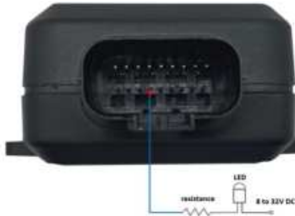
Figure 13. Typical Connection with a LED
