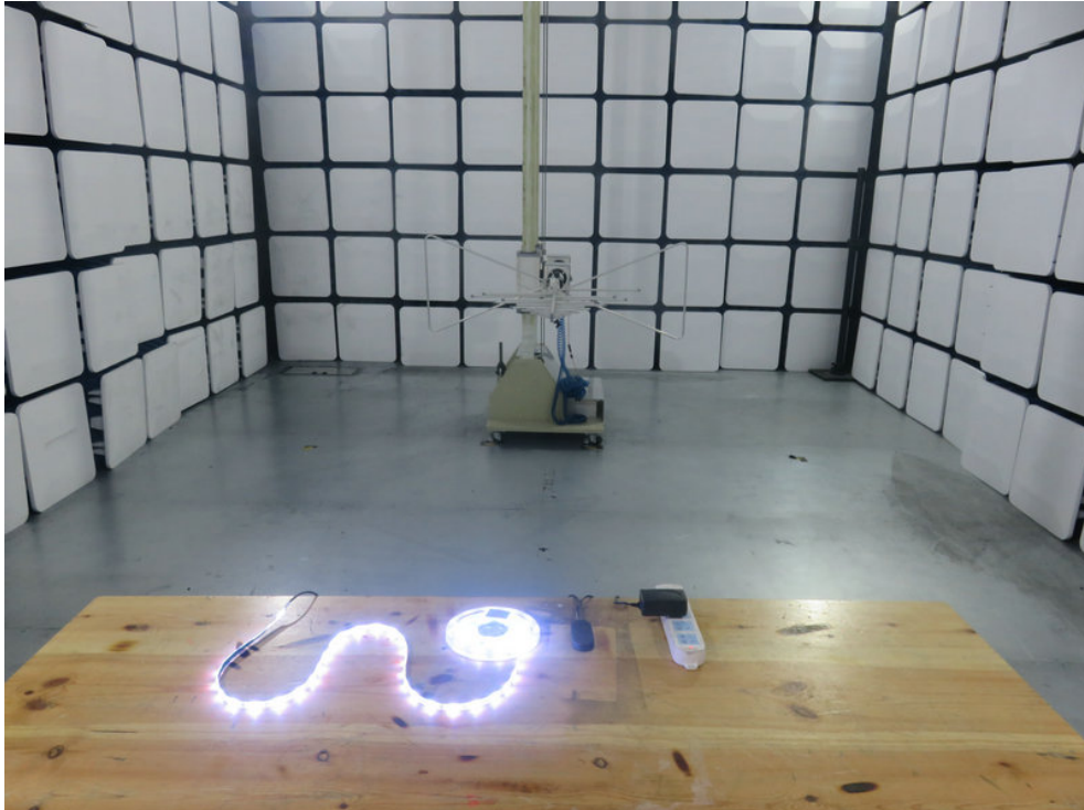
Photo of Radiation Emission Test
