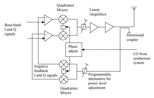
The implementation of the Cartesian loop, involves the use of an integrated Cartesian loop IC operating at the final carrier frequency. The injection signal from the frequency synthesiser is at 4 times the carrier frequency. This is illustrated in the diagram below.
