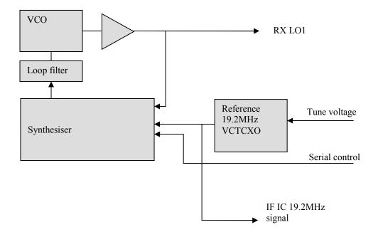
The local oscillator signal (RX LO)1 is at carrier frequency plus IF frequency A 19.2MHz reference signal (fed to a synthesiser on-board the receiver IF IC) enables conversion of the IF signal to base-band I and Q quadrature components.
