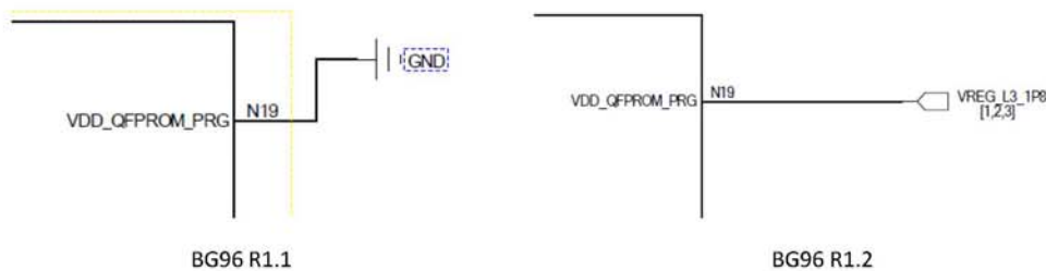
Figure 1: Schematic Designs of BG96 R1.1 and R1.2
