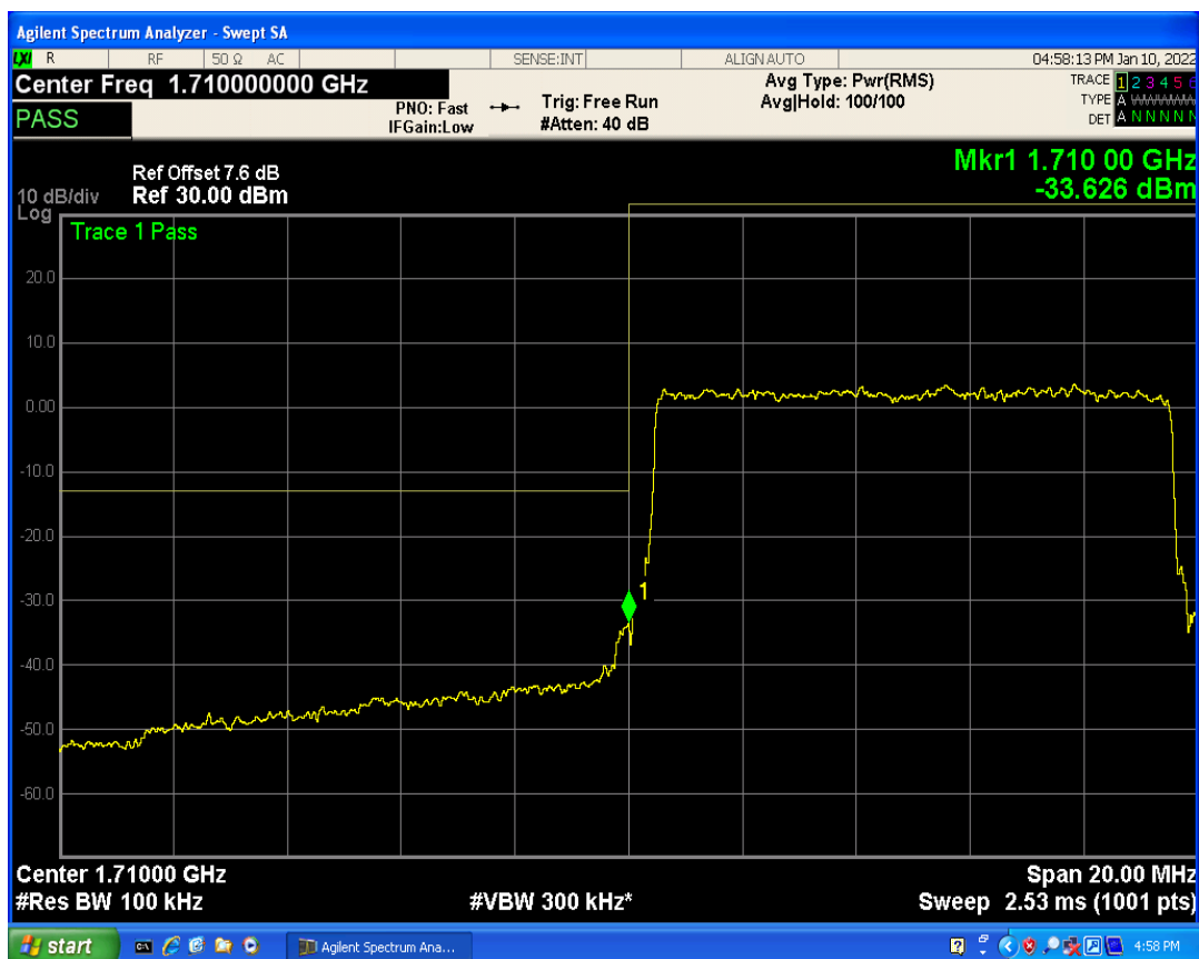
Band66 QAM16 BW=10MHz Channel=132022 RB Size=1 Position=#0
