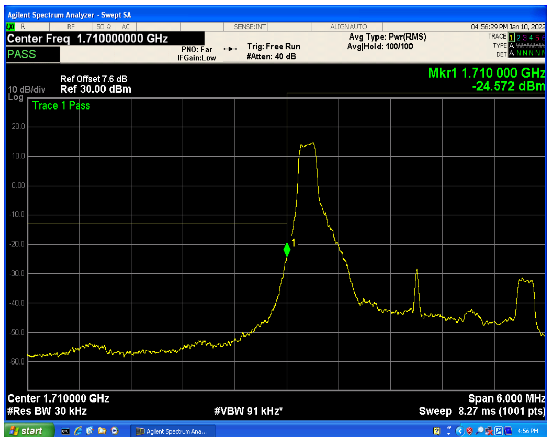
Band66 QAM16 BW=3MHz Channel=131987 RB Size=1 Position=#Max
