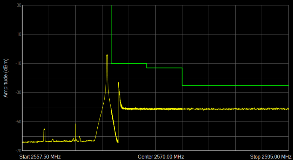
Band7 QPSK BW=10MHz Channel=21400 RB Size=1 Position=#Max
