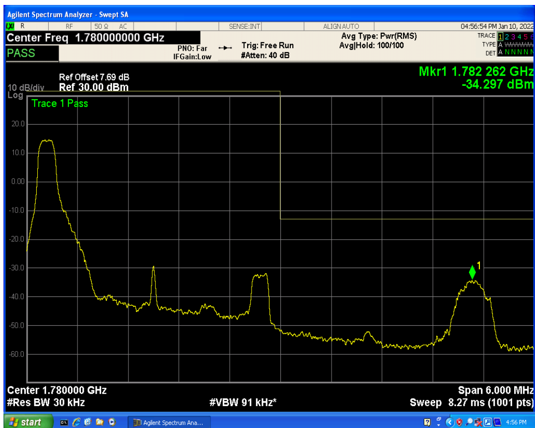
Band66 QAM16 BW=3MHz Channel=132657 RB Size=15 Position=#0
