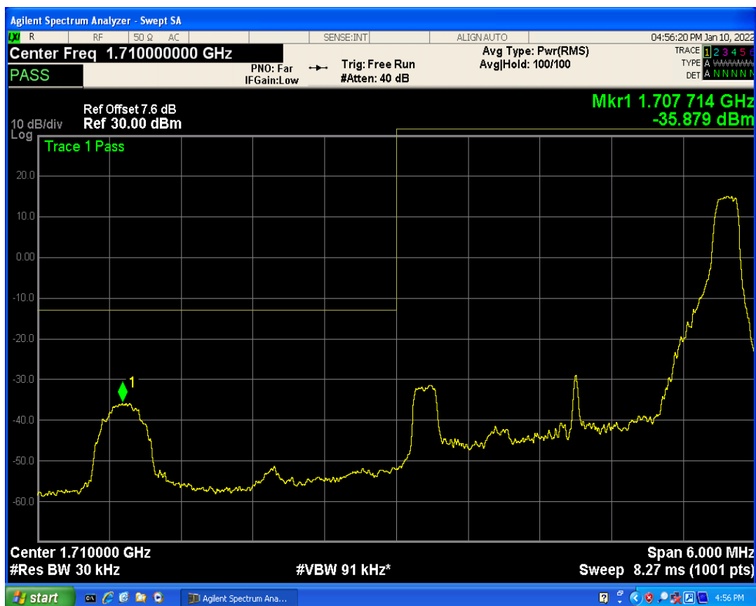
Band66 QAM16 BW=3MHz Channel=131987 RB Size=1 Position=#0
