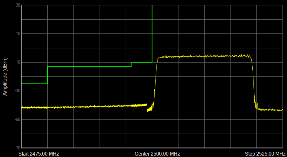
Band7 QPSK BW=20MHz Channel=20850 RB Size=100 Position=#0
