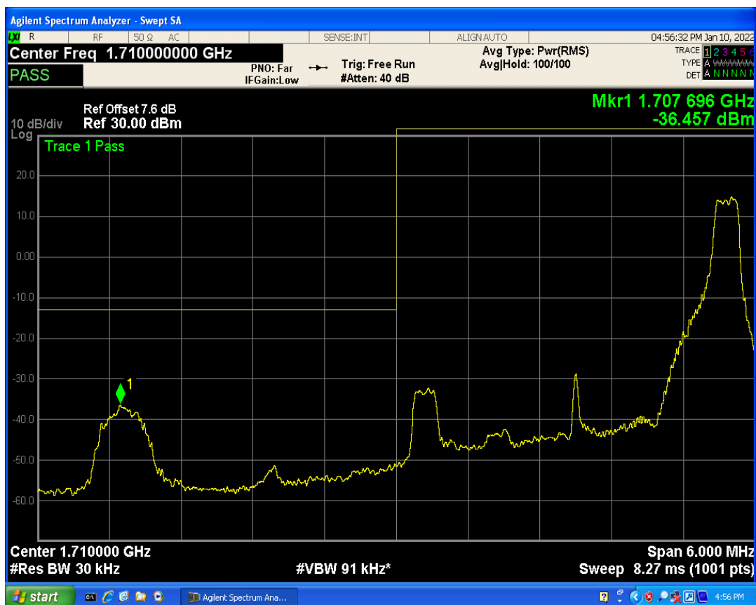
Band66 QAM16 BW=3MHz Channel=131987 RB Size=15 Position=#0
