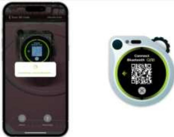
Step 3. After successfully scanning the QR code, the app will navigate to the network configuration page. Select a 2.4GHz Wi-Fi network to connect your Watcher to the internet.
