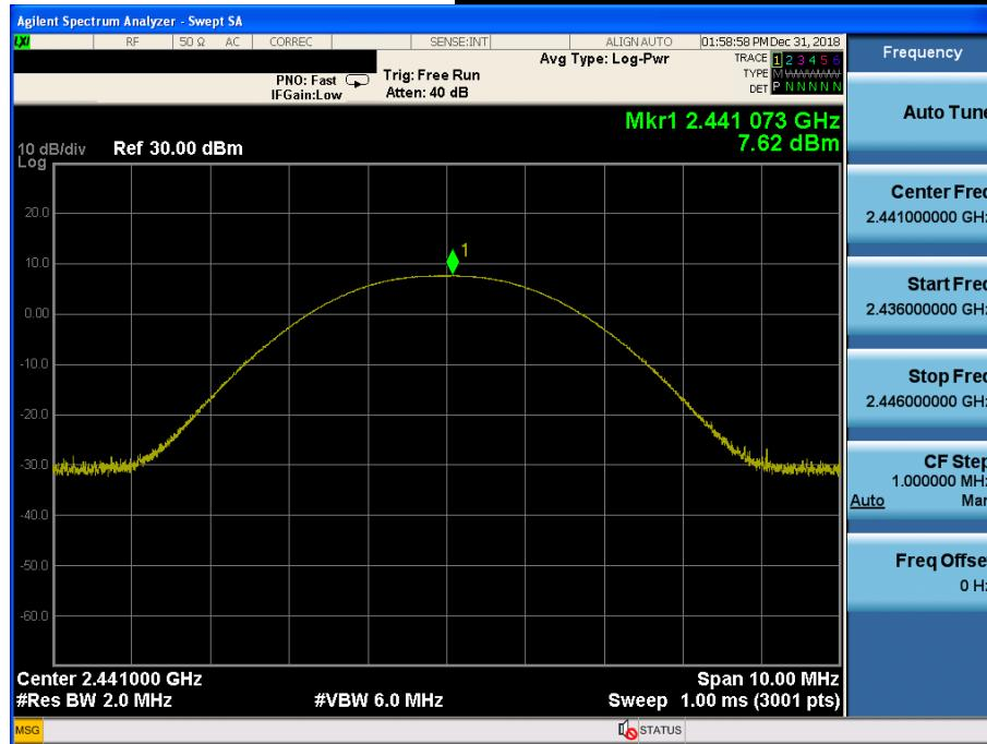
**Peak Output Power****Highest Channel & Modulation : 8DPSK**
