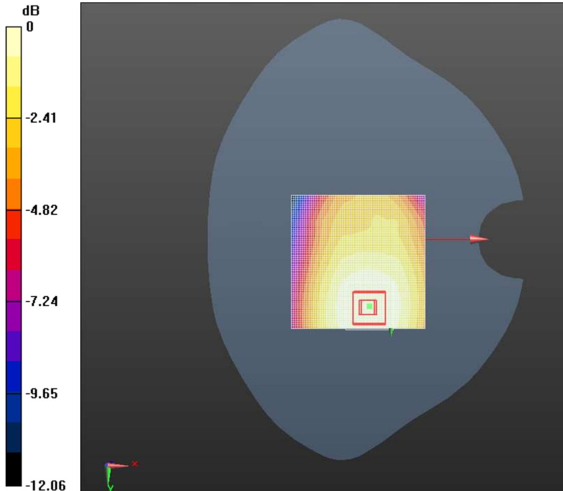
$$0 \text{ dB} = 0.187 \text{ W/kg} = -14.56 \text{ dB W/kg}$$
