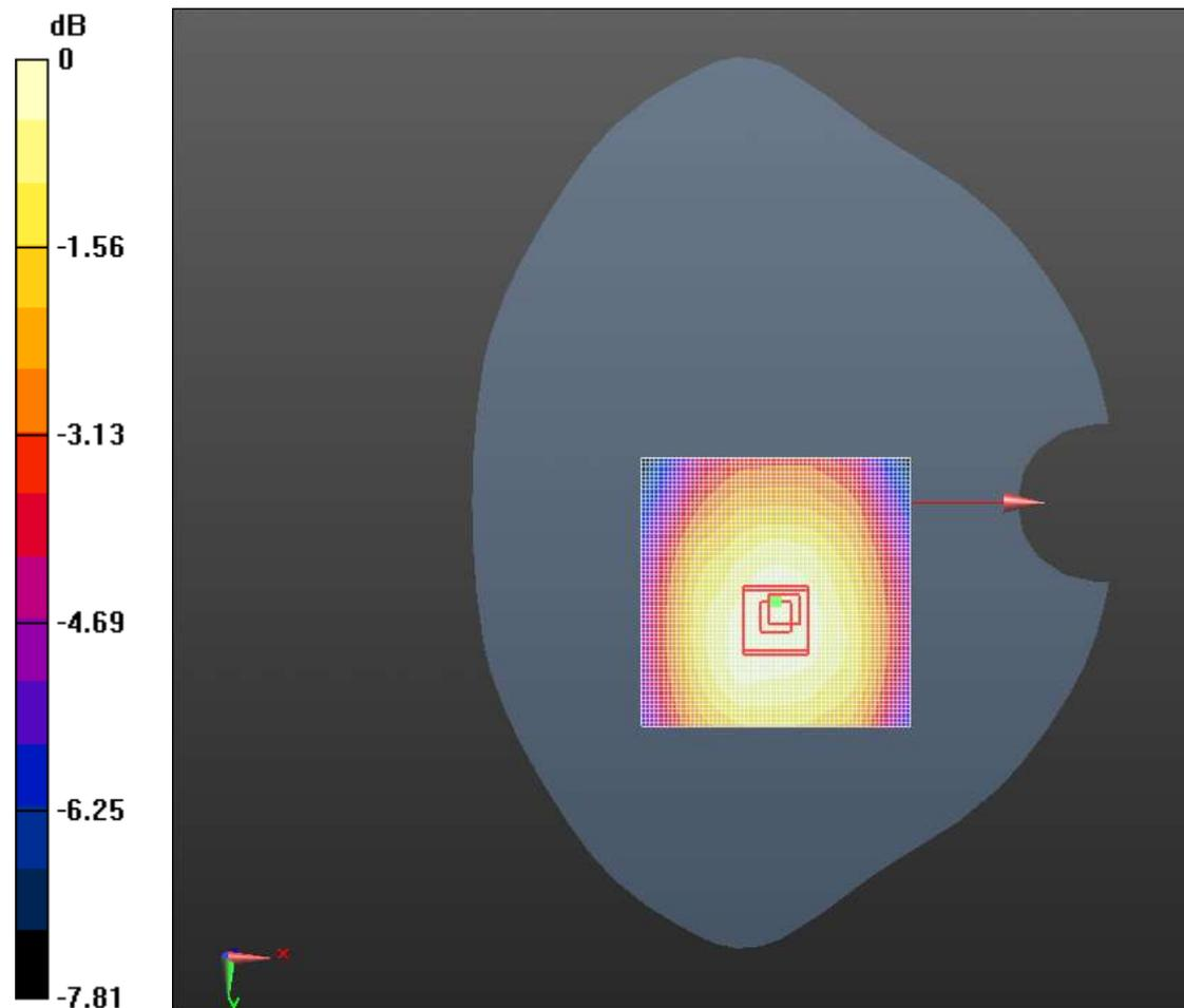
$$0 \text{ dB} = 0.245 \text{ W/kg} = -12.20 \text{ dB W/kg}$$
