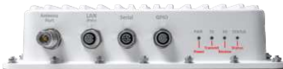
FIGURE 1 - Connector and LED indicators
