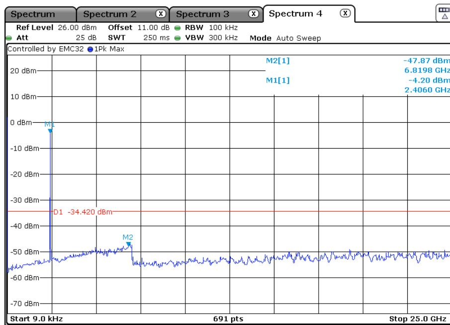
In any 100kHz bandwidth, the Conducted Spurious Emissions from 30 MHz to 25 GHz were greater than 30dB below the peak emission within the band that contains the highest level of the desired power.
