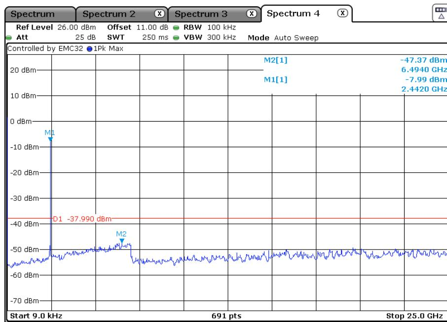
In any 100kHz bandwidth, the Conducted Spurious Emissions from 30 MHz to 25 GHz were greater than 30dB below the peak emission within the band that contains the highest level of the desired power.
