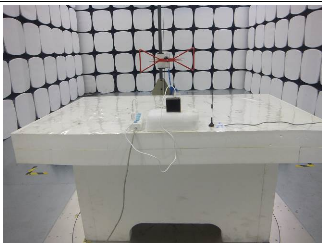
Radiated Spurious Emissions Test Setup Below 1GHz
