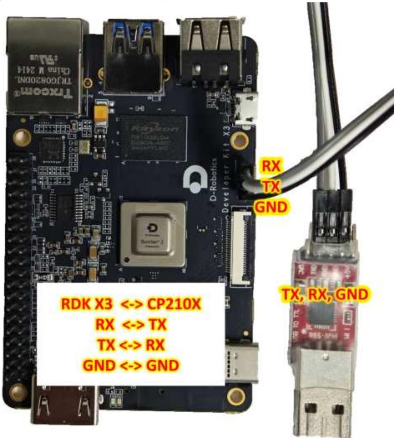
The RDK X3 Module carrier board provides one debugging interface (Interface 15). Hardware-wise, the core module debugging serial port is converted into a USB interface via the CH340 chip, allowing users to perform various debugging tasks using this interface. The parameters of the computer serial port tool should be configured as follows:
