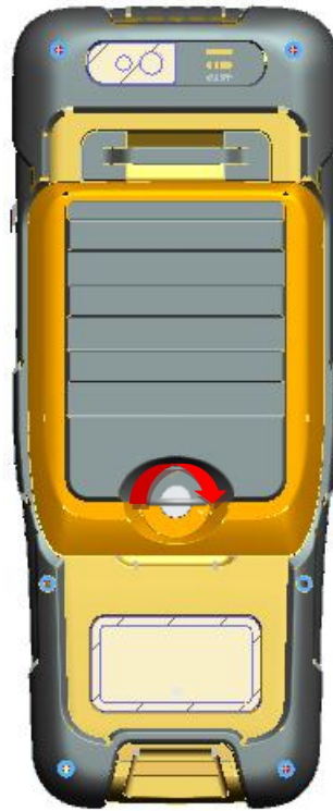
Figure 2.6 Insert the back cover
