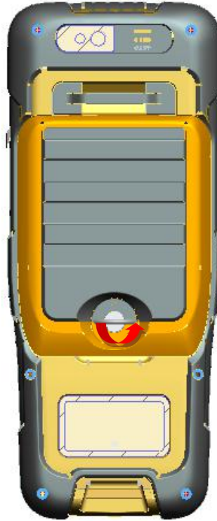
Figure 2.2 Remove the back cover
