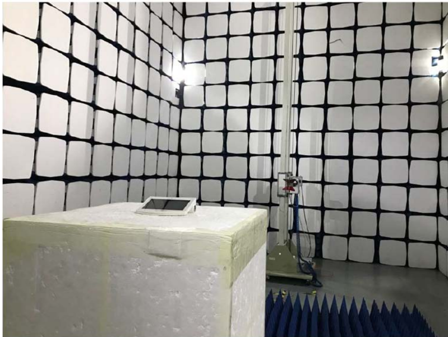
Radiation Emission Test Setup (1GHz to 18GHz)
