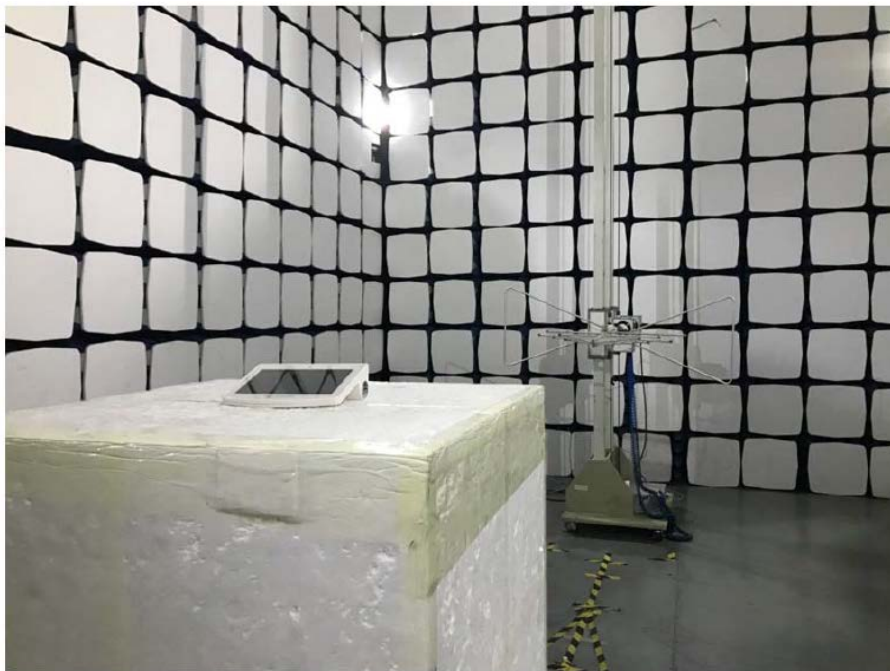
Radiation Emission Test Setup (30MHz to 1GHz)
