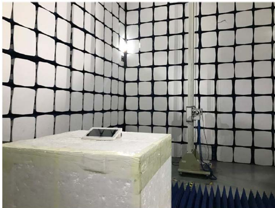
Radiation Emission Test Setup (Above 18GHz)
