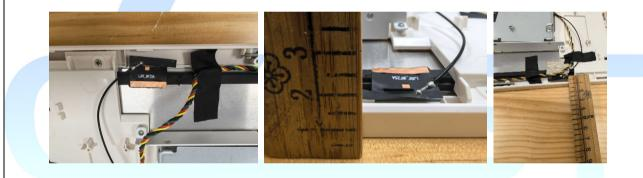
Remark: the distance calculated is the antenna installation location to touch screen, simultaneous transmission not support
