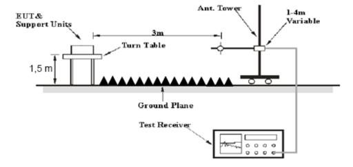
The radiated emission below 1GHz tests were performed in the 10 meters chamber test site, above 1GHz tests were performed in the 3 meters chamber test site B, using the setup accordance with the ANSI C63.10-2013. The specification used was the FCC 15.209, and FCC 15.249 limits.
