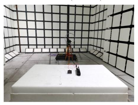
Radiated Emissions View (Below 30MHz) Perpendicular
