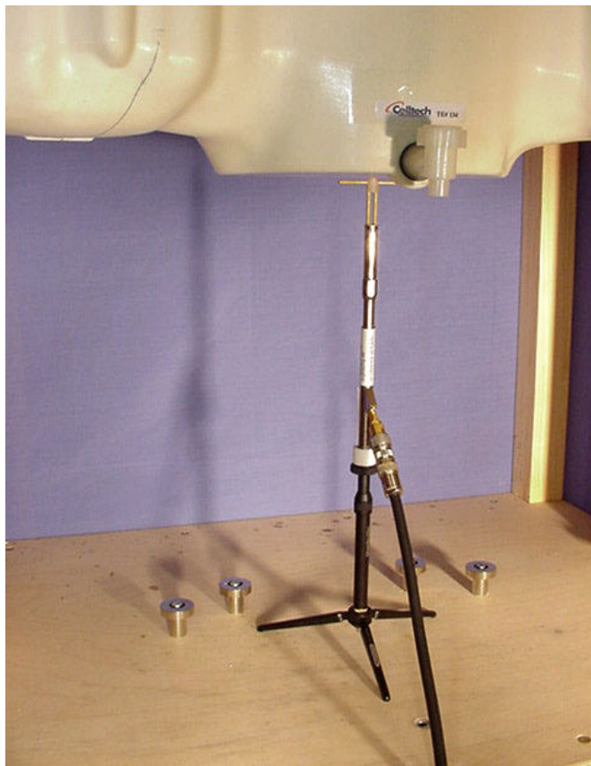
1800MHz Dipole Validation Test Setup
