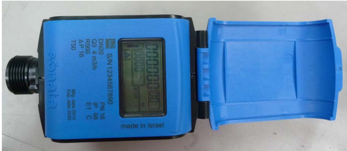
Photograph No.4 “SONATA” LCD under top cover
