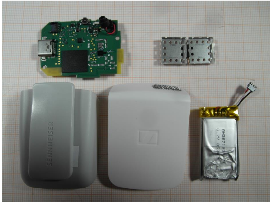
Photo 1: EUT disassembled with battery pack (front view)
