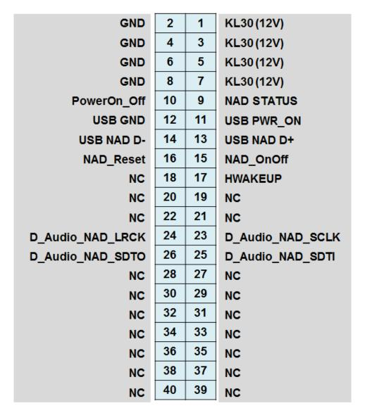
Figure 1. Connector pin arrangement
