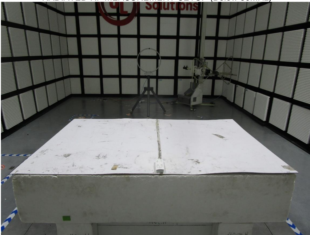
RADIATED RF MEASUREMENT SETUP (Below 30MHz)
