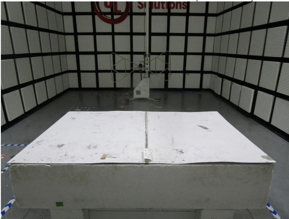
RADIATED RF MEASUREMENT SETUP (Below 30MHz)
