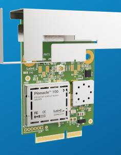
The Pinnacle<sup>™</sup> modem seamlessly incorporates a powerful Cortex M4F controller, full Bluetooth v5 and LTE-M capabilities – all with full regulatory certifications and LTE carrier approvals.
