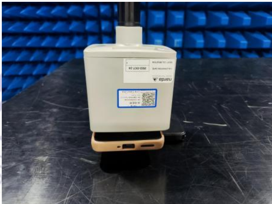
Portable exposure conditions Test Position A (2cm)
