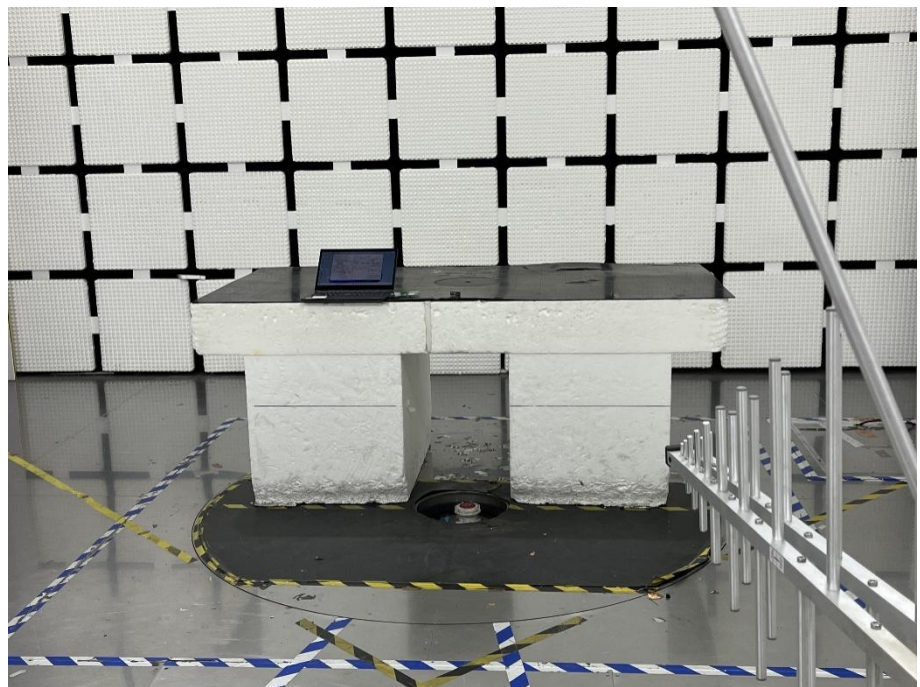
Radiation Emission Test Setup (30MHz to 1GHz)
