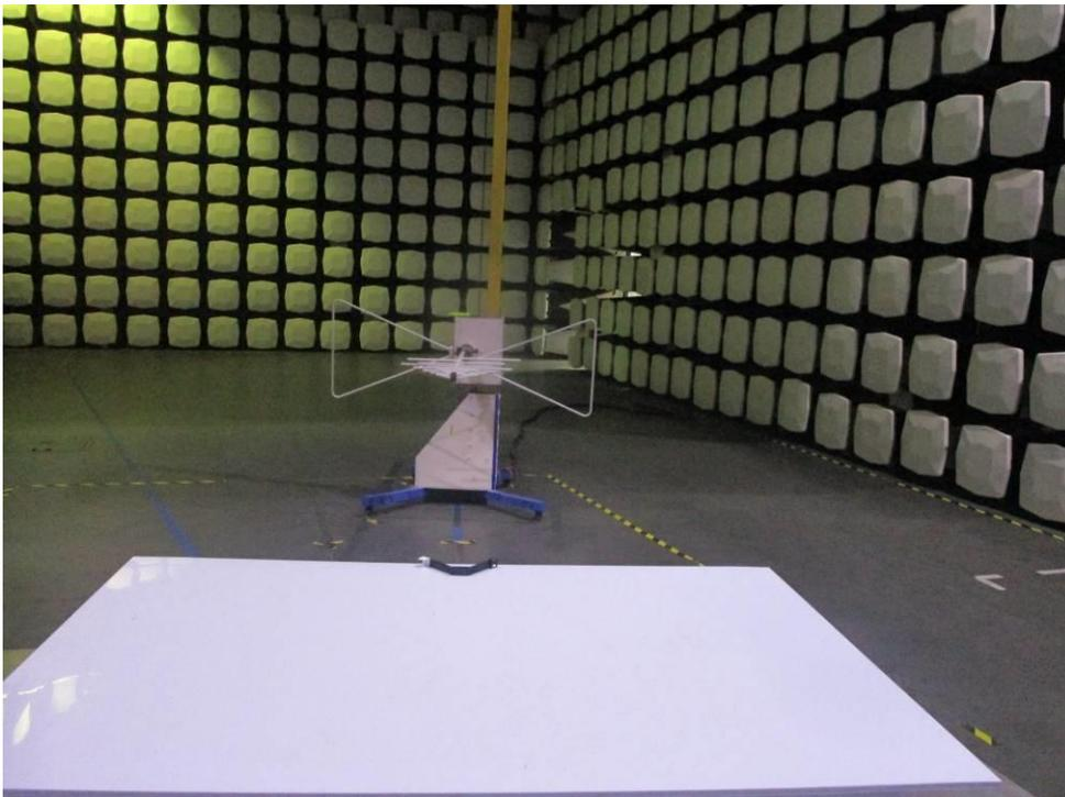
**Radiated Spurious Emissions & Radiated Emissions which fall in the restricted bands (Above 1GHz)**
