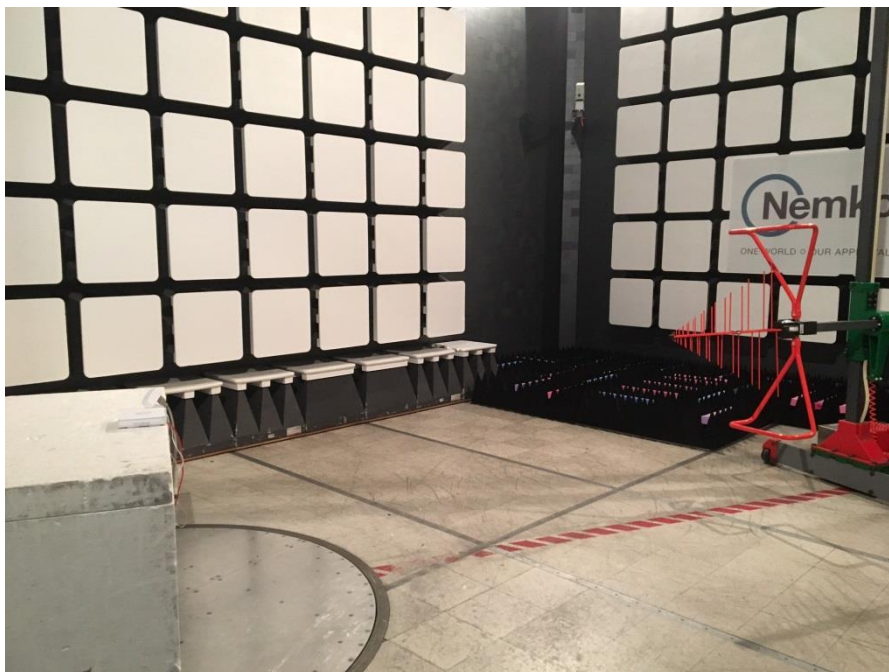
Figure 8.1-17: Radiated – Undesirable (unwanted) emissions setup photo – below 1 GHz
